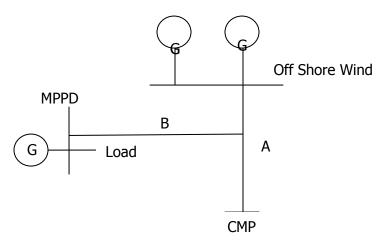
The Off Shore Wind project will connect to the on shore power system, owned and operated by Central Maine Power (CMP), via the subsea cable identified as "A". This will allow power to flow in both directions:
